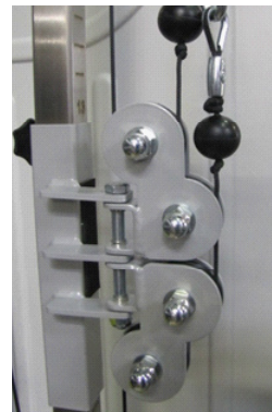
Cable pulleys have to be positioned vertically
