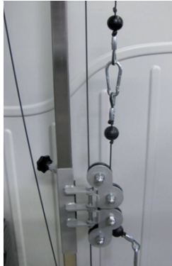
Run the cable upwards through all pulleys
