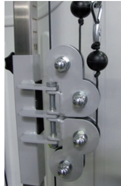
Cable pulleys have to be positioned vertically
